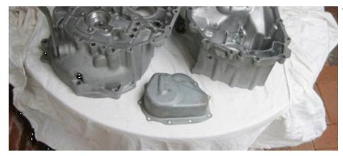
The entire casing was sandblasted using 1mm paving sand, a cheap sandblaster gun from Repco and a small 2.5hp air compressor:
