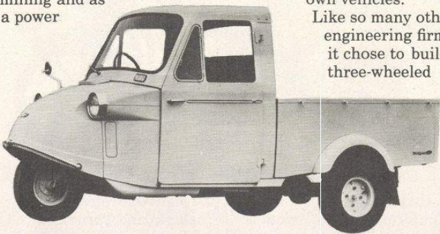
Midget of 1957 was a three-wheel commercial with 540 cm 3
